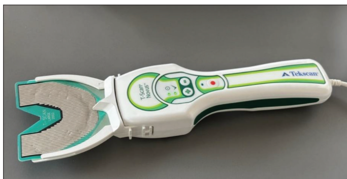
Figure 3. T-Scan Novus (Tekscan Inc., Norwood, MA, USA) handpiece with sensor film
